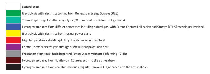
The production of hydrogen thanks to a renewable or nuclear energy source (or by steam reforming of natural gas if the process is associated with a CCUS system) is called "low-carbon hydrogen" and quickly became an environmental and political priority, as we demonstrated earlier. To achieve Green Hydrogen, we therefore need RES, water and electrolysis.
