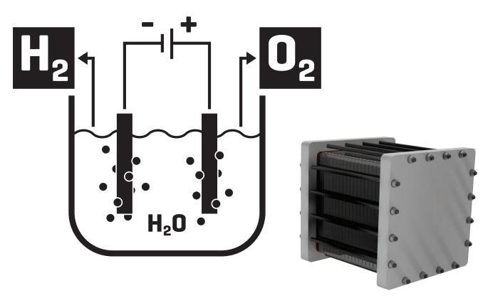
While the two precedents are quite easy to understand, electrolysis process is more complicated and we need to focus on how it works. While there are more and more types of electrolysis being developed, two models are commonly differentiated: alkaline electrolyser and proton exchange membrane (PEM). The creation process of hydrogen (or, more precisely, a mix of hydrogen and oxygen) is slightly different from one type to another but it is commonly accepted that:
