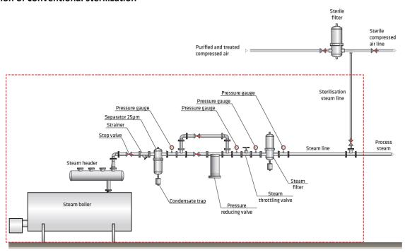
Scheme of a conventional sterilization in place system. All the equipment surrounded by red line is required to perform sterilization of the filter housing in the upper right corner. Such a fixed steam distribution line connects steam generator to every filter.
