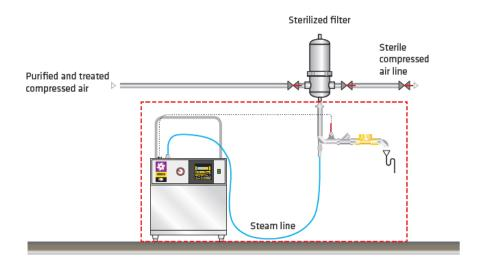
Scheme of a new Mobile Steam Sterilizer connected to a filter. After sterilization cycle is completed flexible hose for steam distribution is disconnected from the filter and complete sterilizer (equipment surrounded by a red frame) can be moved to another location.
