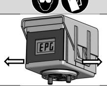
The direction plate should be rotated so that the arrow on the bottom of direction plate points in the direction of air flow through filter.
