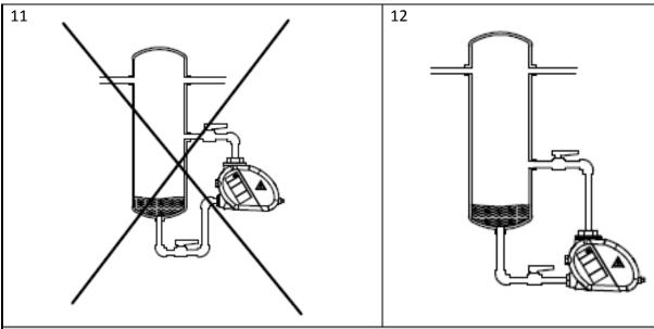
In case there are problems with inflow, it is necessary to install a venting line (12). In this case back connection is used as inlet and upper connection is used as air ventilation. Venting line must never be installed as it is on pictures 9, 10 and 11.
