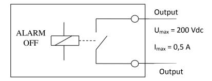
The switch is closed when CDi operates normally and it is open when CDi is in alarm mode or when power is disconnected.
