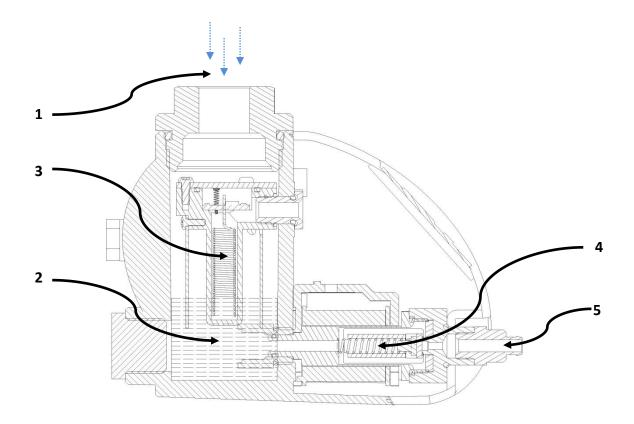
Condensate flows through inlet connection (1) and accumulates in the reservoir (2). Sensor (3) is measuring condensate level. When reservoir (2) is detected full, sensor (3) sends signal to electronic board. Electromagnetic valve (4) is than opened to discharge accumulated condensate through outlet connection (5). When reservoir (2) has been emptied, the valve (4) closes back without any losses of compressed air.
